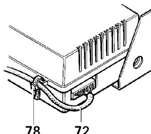
For strain relief, secure control panel cable (72) on the control electronics by means of enclosed cleat (78).
